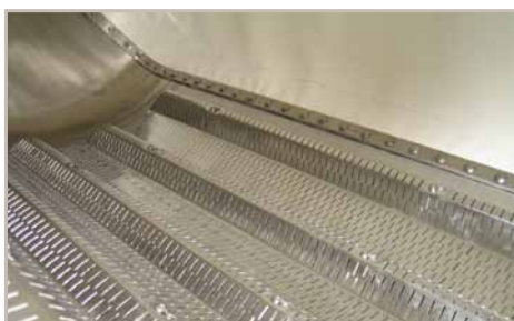
connected draining channels, electropolished
