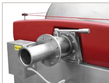
overfilling signalisation, axial filling valve
